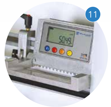
Electronic vertical measuring display Mecedor digital para posición vertical
